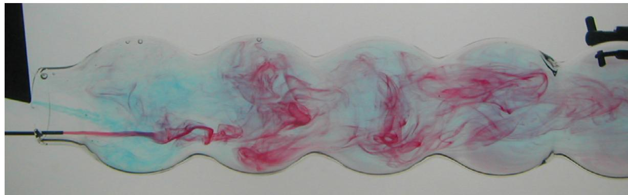
Dye flow visualization of evolution of wingtip vortex in sinusoidal tube. Blue color dye represents wing tip vortex, whereas red color represent freestream flow enters the tube.
