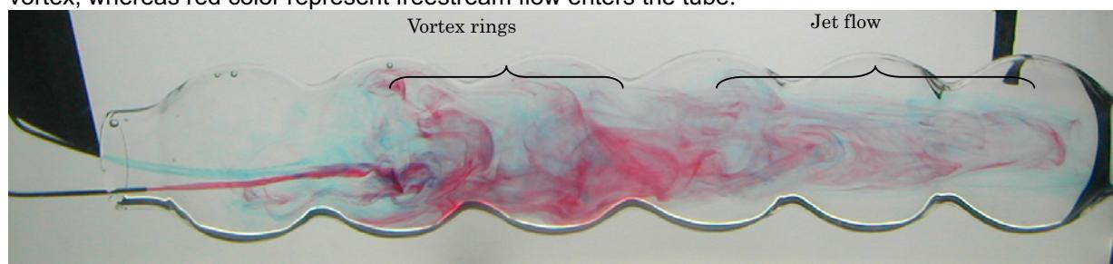
Evolution of vortex in sinusoidal tube. The jet flow patterns downstream after the fourth lobe is clearly visible.
